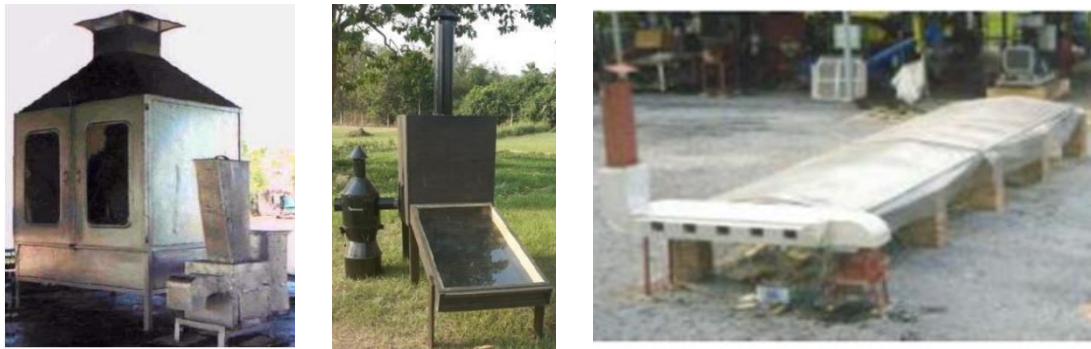
Figure 5: (a) and (b) Hybrid solar biomass cabinet dryer (c) Hybrid solar biomass tunnel dryer
