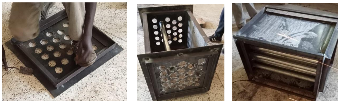
Figure 25: Heat exchanger fabrication and assembly
