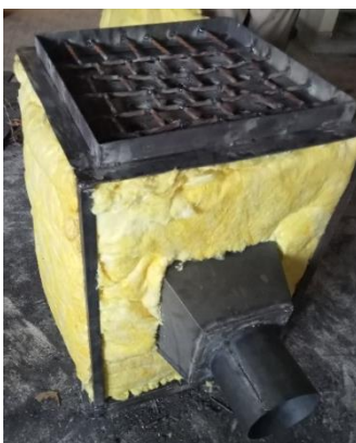
Figure 26: Insulation of heat exchanger
