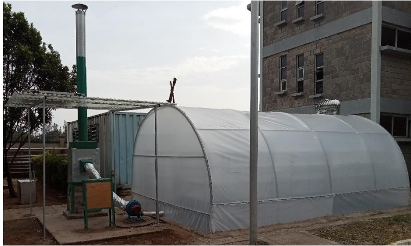
Figure 30: Complete assembled Hybrid solar biomass greenhouse dryer
