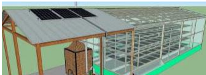
Figure 3: Hybrid solar biomass solar dryer
