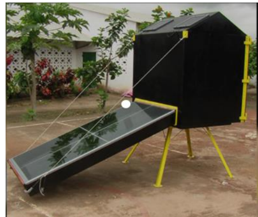
Figure 2: Solar box dryer
